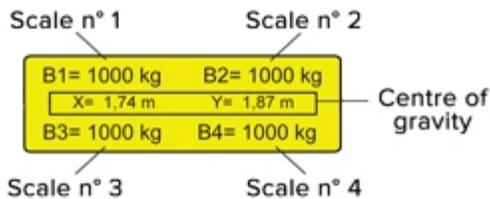
Suitable for creating wheel weighing and static axle weighing systems, or to weigh objects with various resting points. Ideal for weighing and calculating the centre of gravity coordinates of the vehicles, trucks, airplanes, containers, etc. Simultaneous display of the weight of each connected platform and of the sum. CE-M approved (OIML R-76 / EN 45501).
