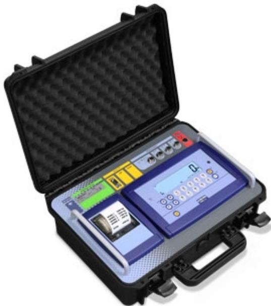
Multifunction digital weight indicator in Rack version complete with 4 connectors for linking the platforms, built-in rechargeable battery, battery charger, thermal printer, time/date and case. It is particularly suitable for vehicle weighing applications. CE-M approvable (OIML R-76 / EN 45501).
